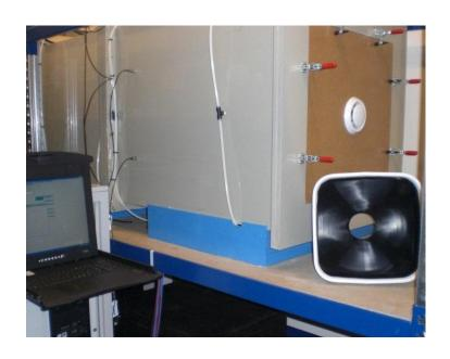
Laboratory investigation into the market leading vane anemometer & hood assembly measurement accuracies
